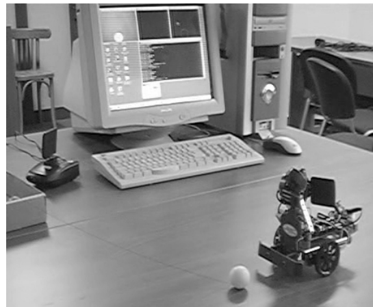
Fig. 7. A simple robot following a ping-pong ball
