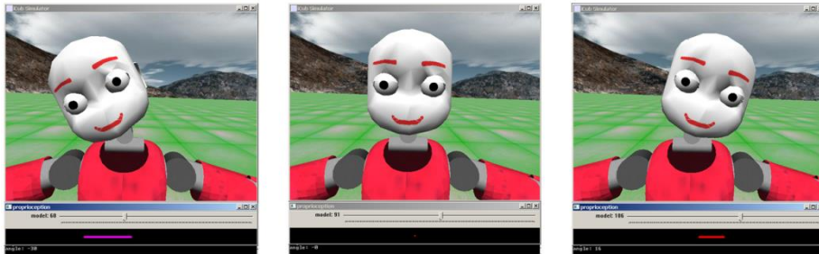
Fig. 4. Proprioception mechanism provides simplified body model (pink color indicates head gradient to the right, red color to the left – from robot's point of view)
