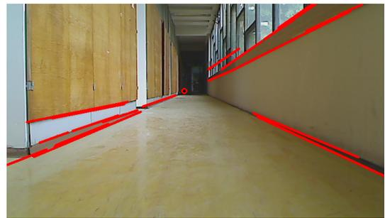
(b) Horizontal and vertical lines are removed from vanishing point estimation.
