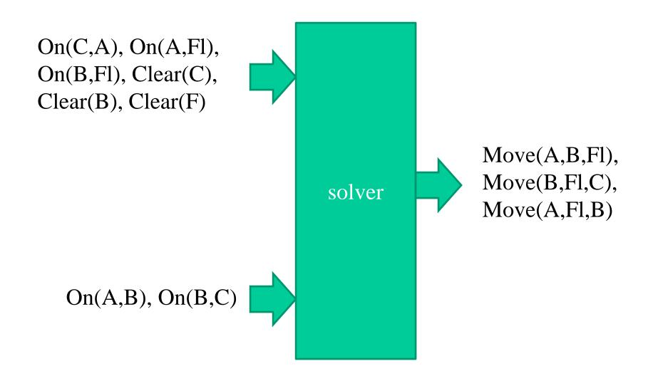
The solver tries to put various instances of the STRIPS rules into a tree structure that connects the initial state with goals.
