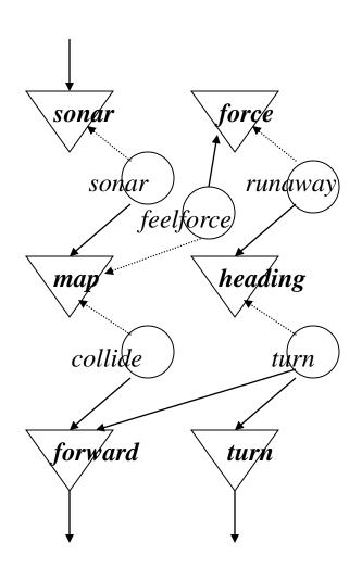
Let us concern that rotation of robot provides feed back to sonar measurement what has impact to heading of robot. More the robot rotates from colliding direction, less rotation is ordered in *heading*.
