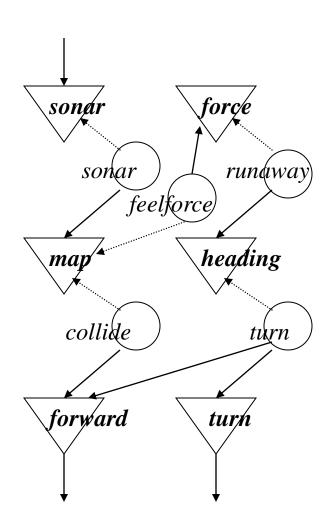
Finally *turn* transform the direction to wheel rotation
