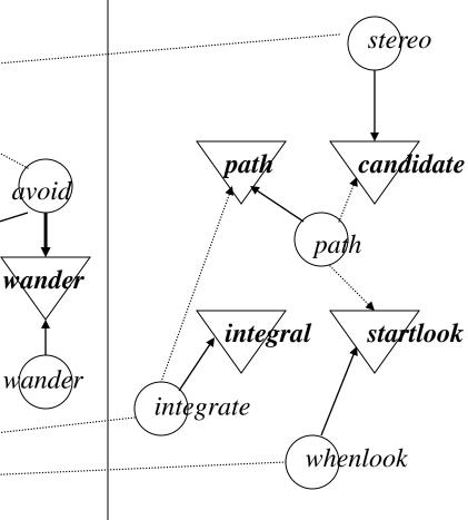
However it is direction relative to robot this integral helps to calculate its absolute value which will not change when robot rotates
