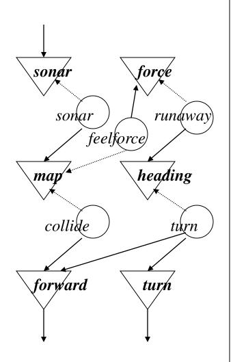
Thus the robot goes ahead until it meets obstacle. The it starts to rotate until no collision is threatened. Than it goes straight again.
