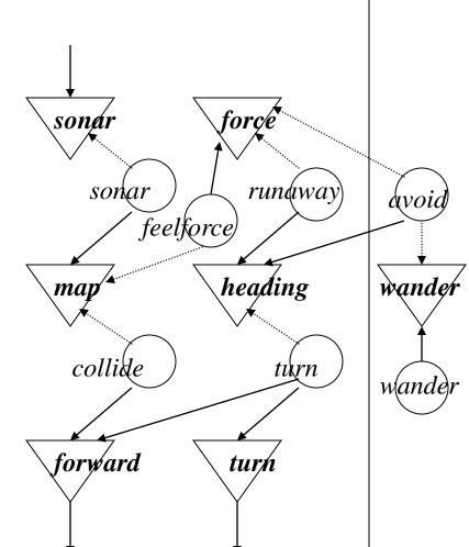
And agent avoid checks if there is no acute obstacle avoiding and if no, it writes the proposed angle into heading as if the angle would the right angle for obstacle avoiding.
